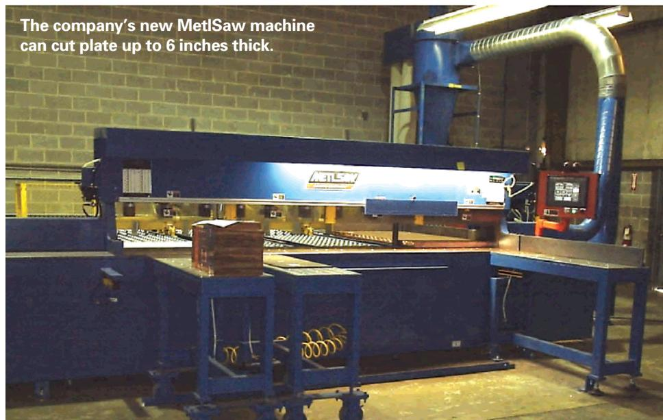
The company's new MetSaw machine can cut plate up to 6 inches thick.
